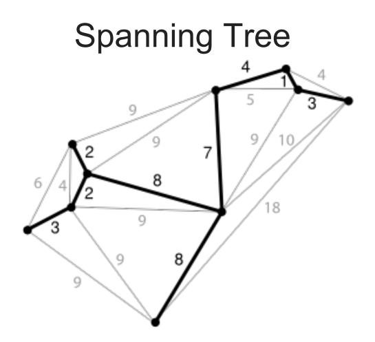
Points – represent switch in network Numbers – represent cost to transmit to next switch Switch – each switch has computers attached
